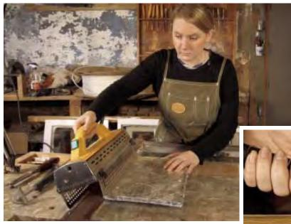
run a safety razor back and forth over the surface of the glass before polishing it with a cloth.
