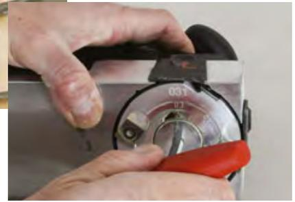
**Drawbacks.** Like the Paint Shaver, the Metabo is outfitted with side cutting blades. These blades appear capable of stripping paint off the undersides of clapboards but in practice they are ineffective; their cutting depth is extremely shallow and there doesn't seem to be any way to adjust them. The owner's manual was no help in this regard. All of the tool's blades tended to gum up with old paint, but they were easy to clean using the miniature scratch awl included as part of the kit.
